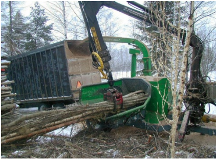
Figure 67. Small tree chipping with disc chipper (Kesla) at a road side (VTT)
